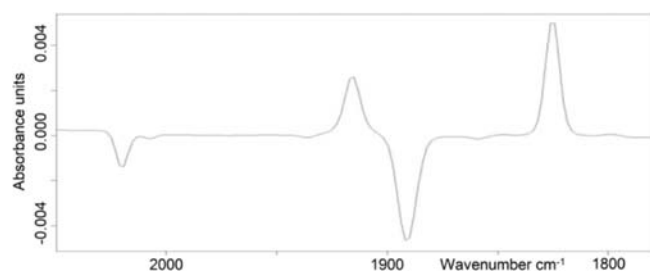
Figure 2. FTIR difference spectrum of \sim 10^{-3} M (L_{OEt})Re(CO)_3 ( 1 ) in c\text{-C}_5\text{H}_{10} at 200 K after exposure to 266 nm radiation.
